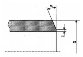
Figure 1 — Tube end bevel
